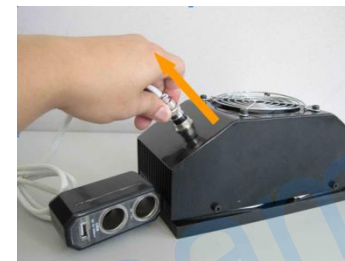
② Anticlockwise rotate to unlock
